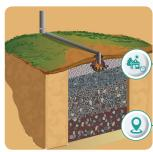
What: A dug out pit filled with graded stones and gravel
