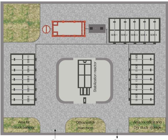
Figure 10: Layout for FSTP Based on Unplanted Drying Beds
